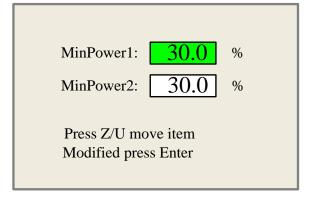
When "Z/U" key is pushed, the green block can move up and down to denote the changing item, then "Y+/-" keys and "X+/-" keys can be used to change the value.
