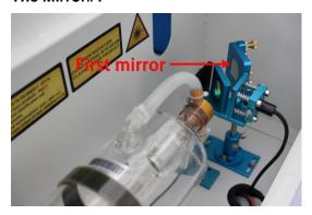
The mirrors are easily get dirty. And this will reduce the efficiency of the laser beam. Meanwhile, laser energy absorbed by the mirror may cause heat and destroy the mirrors too. For the first mirror, you can clean them directly.
