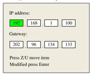
Push "Z/U" key to move the changing item, then push "X+/-" keys and "Y+/-" keys to change the value, when all the IP value and the Gateway value are changed, push "Enter" key to validate the change, or "Esc" key to invalidate the change.
