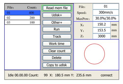
When showing this menu, the system would read the memory file firstly, the file name and the work times would be listed in the area, and the selected file is previewed in the bottom right area. "Y+/-" keys could be used to move the cursor on the file name list. When the cursor is on a target file name, presses the "Enter" key, the selected file will be previewed on the main interface, and then if "Esc" key is pushed, the preview will disappear.
