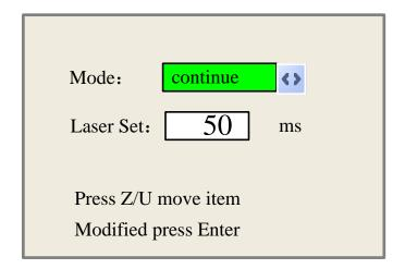
Push "Z/U" key to move the green block, and when the green block is on the "Mode" item, push "X+-" keys to select the anticipant value, "Continue" or "Manual". When "Continue" item is selected, then the "Laser Set" item is not valid, on that time, push the Laser key to splash the enabled lasers, and when Laser key is loosed, then the lasers will finish splashing. When the Mode item is "manual", then pushing the Laser key one time, the enabled lasers will splash a fixed time.
