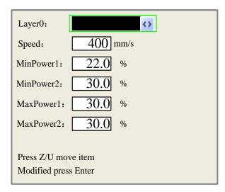
User can push "Z/U" Keys to move the green block on the intent parameter, then he could change the parameter if needed. "OK" to validate the change, and "Esc" to invalidate the change.
