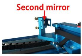
Make sure the power of the laser machine is turned off while cleaning. The 2<sup>nd</sup> mirror is installed on the left side of X rail. For the second mirror, you can clean them directly.
