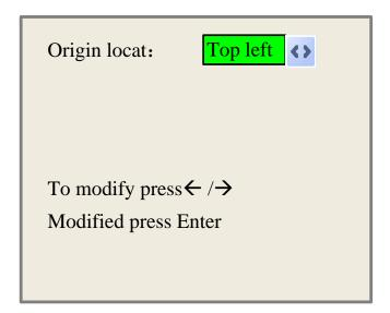
There are four entries to be selected: Top Left, Top Right, Bottom Left and Bottom Right. When one is selected, the previewed graph on the screen would be enantiomorphous based on X or Y direction.
