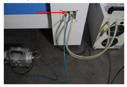
The input voltage must correspond (AC 230V 50/60 Hz or AC 115V 50/60 Hz) - see information label beside the connection socket.
