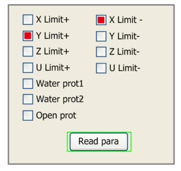
This interface shows some system input information, such as limiter status, the status of the water protecting, and the status of the foot switch etc.. When the input is validated, the color frame will be red, otherwise it's gray.
