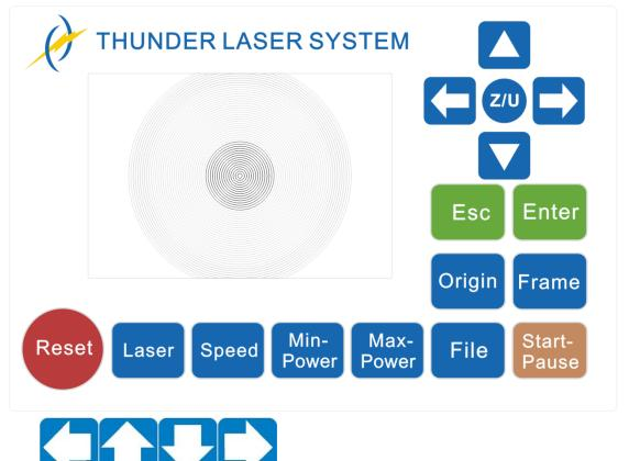
Arrow buttons: control the movement of the laser head. (also can be used to change the parameters in the control panel)
