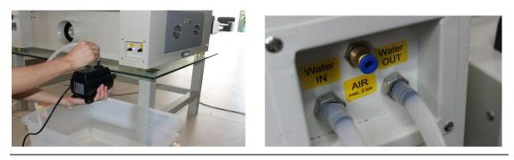
Get through the water chiller or the water pump , and turn on the main power. Check the water chiller or pump to work (If normally work, the green light will light or water will flow from the pipe).
