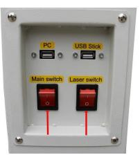
If all covers are closed, immediately after being switched on, the device starts the referencing process. When the referencing process is completed correctly, an acoustic signal sounds and the device is ready for operation. The operation panel will display the home screen when the laser is completed resets.
