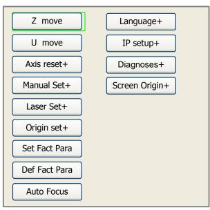
Press up and down arrow keys to move the green block to the anticipant item, and then push the "Enter" key to display the sub menu.
