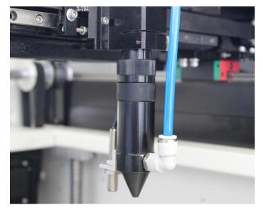
4" laser head owns a longer focal distance than 2" standard head, thus for cutting thick material, it makes the cutting edge more smooth and straight.
