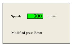
Push the "X+/-" Keys to move the cursor in the numeral area, and push the "Y+/-" keys to change the value, then push the "Enter" key to save the change, push the "Esc" key to invalidate the change.
