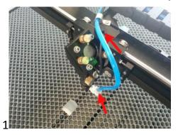
Remove the air pipe and the autofocus
