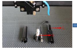
①4" laser head②install the mount mouth to the 4" head
