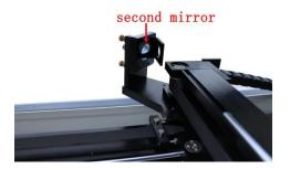
Make sure the power of the laser machine is turned off while cleaning. The 2<sup>nd</sup> mirror is installed on the left side of X rail. For the second mirror, you can clean them directly.
