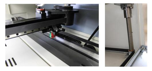
It is suggested to add lubricant oil (or Rust Preventative Grease) to the rails/screws at least every two weeks.
