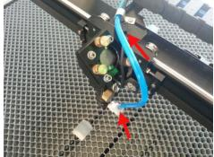
Reinstall the air pipe and auto focus interface.
